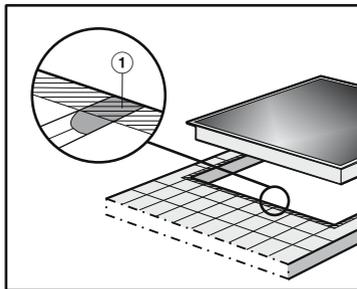
► Grout lines ① and the hatched area underneath the hob frame must be smooth and even. If they are not, the hob will not sit flush with the worktop and the sealing strip underneath the hob will not provide a good seal between the hob and the worktop.
